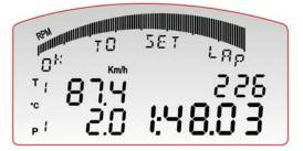
• Once lap marker is set, GPS lap timer setting procedure is over and the display shows a confirmation screen ("GPS MARKER END"). This screen appears only if the procedure has been successfully completed.
